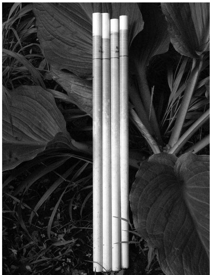
IRIS tubes provide a new way for soil scientists and wetland professionals to identify reduced soil conditions.
