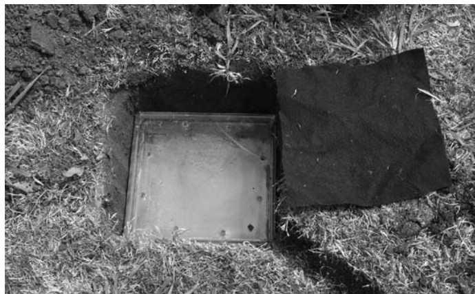
Installation of a glass block lysimeter for collection of leachate at a depth of six inches.
